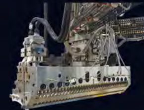
1000 mm. Flat Die and Feed Block 3/5 Layers
