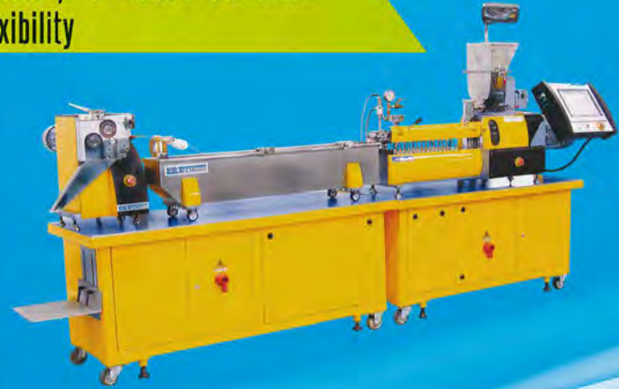
16 mm Twin Screw Extruder with downstream Water Bath and Pelletizer
